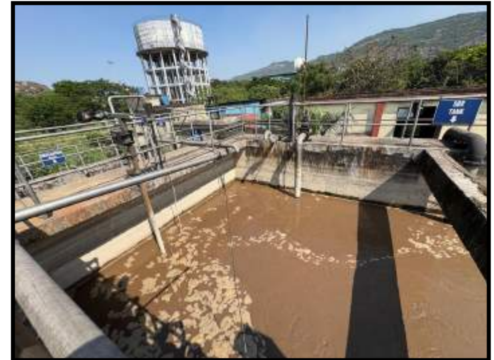
Fig. 5 Flash mixer & Floccutlator tank
